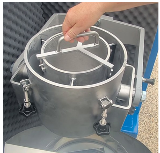
ball and rod mill drum with lifting tool
